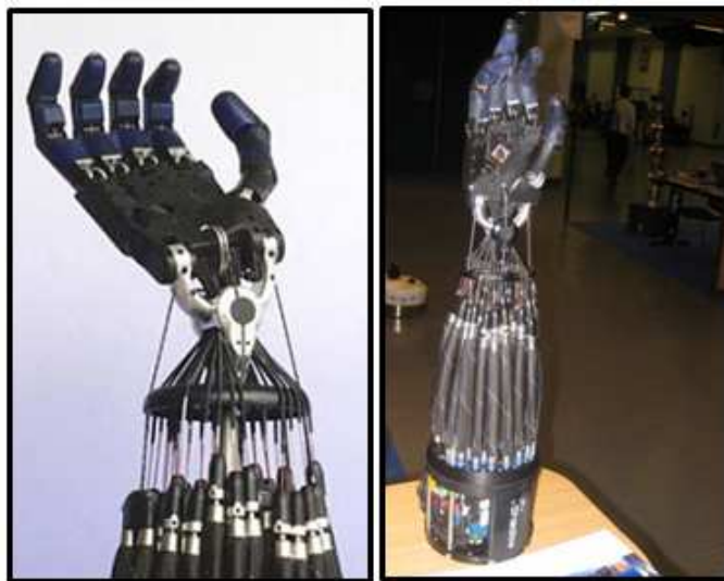
Fig. 6. The Shadow hand actuated with air muscles
