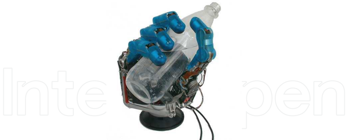
Fig. 9. The DLR hand with four dexterous fingers and a self-contained structure
