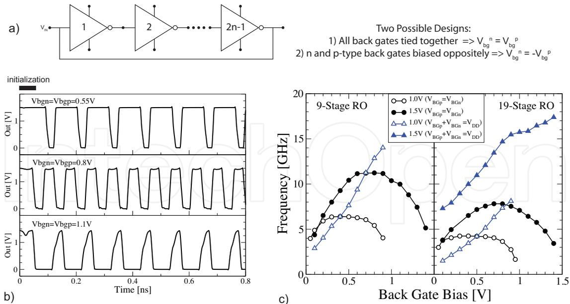
Fig. 11. a) Simple ring oscillator becomes a versatile VCO in the IDDG implementation based on back-gate biasing of inverters ( $L=50\text{nm}$  and  $W_p/W_n=2$ ) b) The transient response of the VCO to various control biases when  $V_{bg}^n = V_{bg}^p$  c) The proposed control characteristics of the VCO in single and dual control schemes for two different sizes of the rings
