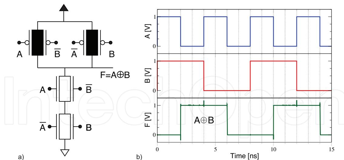
Fig. 17. a) DG XOR circuit with 4 IDDG-MOSFETs, two of which are high  $V_T$  (filled black) and b) the simulated output of this circuit
