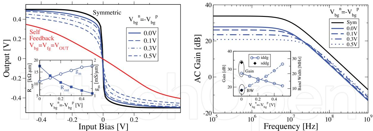
Fig. 3. a) The simulated DC response of the tunable DG-CMOS pair for various joint back gate biases ( $V_{bg}^n = -V_{bg}^p$ ). The amplifier gain changes with the back gate bias and b) AC gain analysis
