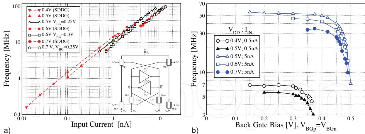
Fig. 12. a) (inset) the switched-current ICO circuit built using IDDG MOSFETs ( $L=50\text{nm}$  and  $W_p/W_n=2$ ) and a latch, and its ICO response. b) The same circuit can also operate as a VCO circuit using back-gate biasing, albeit with a lower sensitivity. Note that the ICO response is extremely linear and spans for orders of magnitude even on a log-log scale
