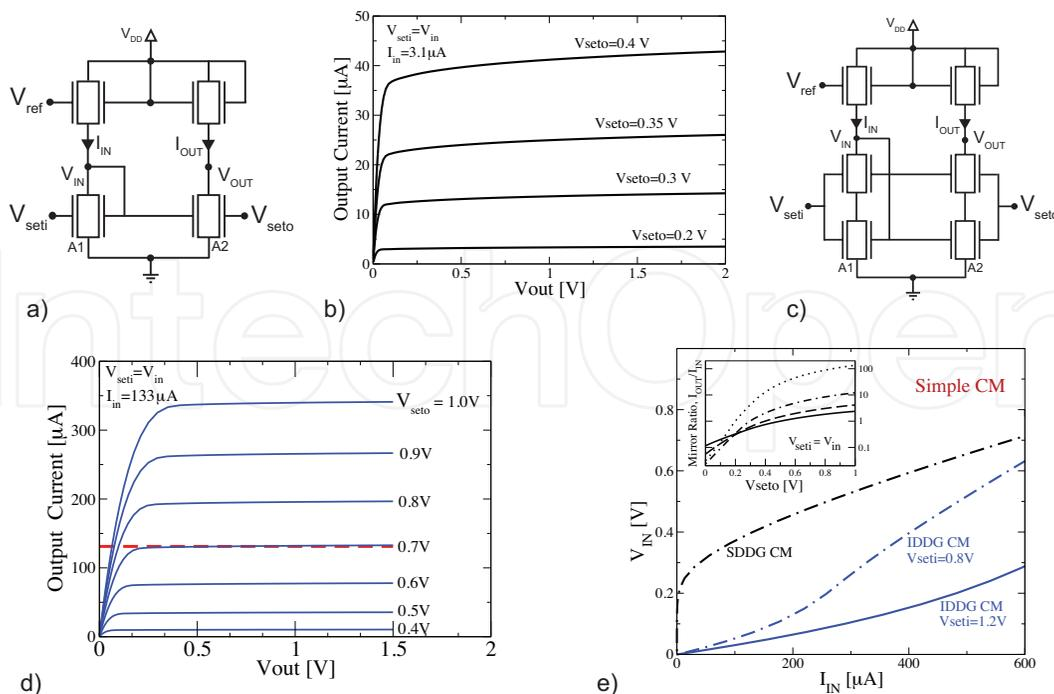
Fig. 4. a) simple DG current mirror and b) the simulated output I-V response as a function of tuning voltage  $V_{set}^o$ . The output impedance is low due to short channel effects c) The improved DG cascade current mirror d) The dependence of the I-V response of the cascade current mirror on  $V_{set}^o$ . e) Comparison of the required voltage across the input of the simple CM in three configurations: SDDG (no back gate control) and IDDG with two different back gate voltages
