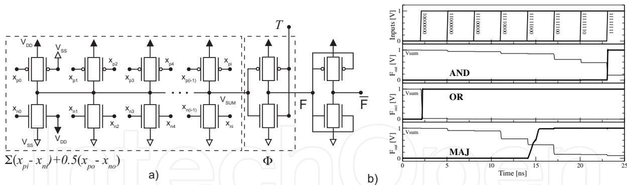
Fig. 18. a) A static-weight threshold logic gate designed using DG-CMOS devices with a minimalist input block and a tunable gate threshold, and b) its simulated logic functionality
