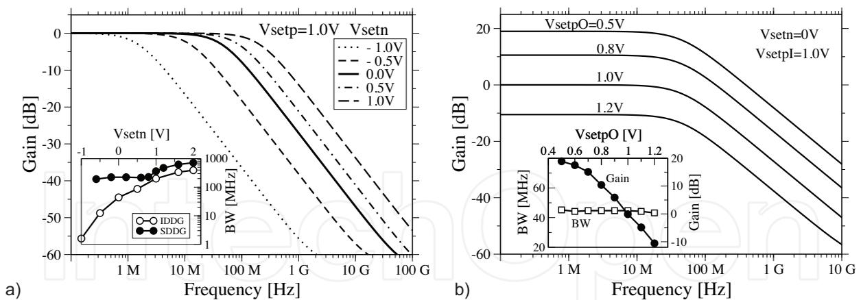
Fig. 9. a) Simulated BW of the balanced integrator for  $C=1\text{pF}$ . The inset shows the extracted tuning range for the same figures in the SDDG and IDDG cases b) Simulated gain tuning of the integrator for  $C=1.0\text{pF}$ . The inset shows there is no trade-off between the BW and the gain in this current-mode circuit.
