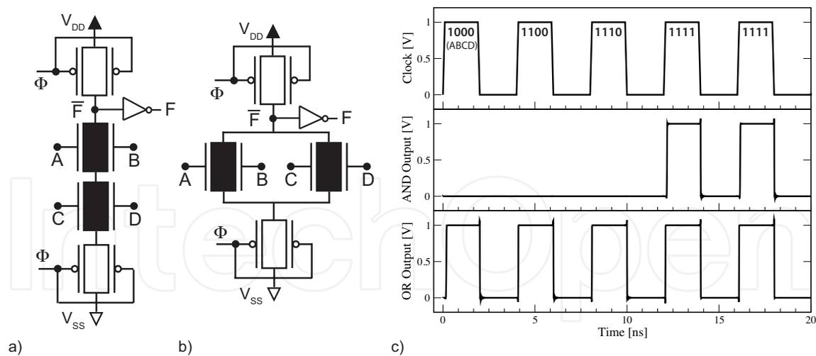
Fig. 16. High- $V_T$  threshold DG-MOSFETs (filled symbols) is used in the logic kernels of the ultra-compact a) 4-input domino F=AND logic gate and b) 4-input domino F=OR logic gate. c) The corresponding timing diagrams obtained from SPICE simulations verifying correct operation as recorded at the non-inverting output (F).
