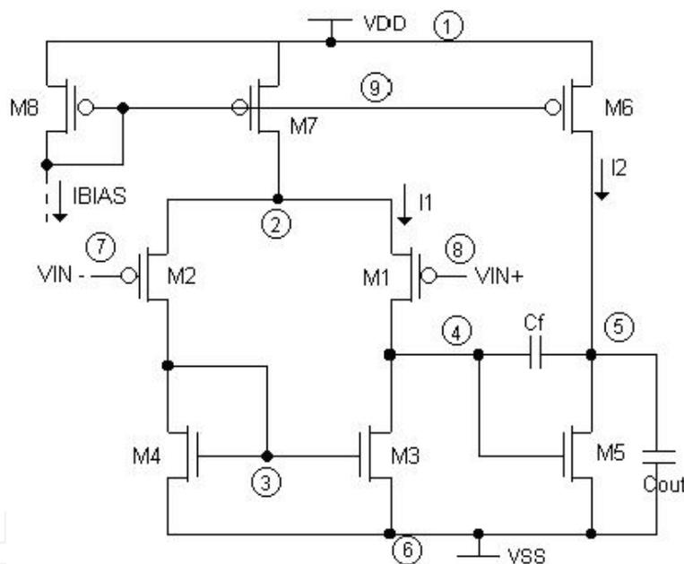
Fig. 1. Schematics of a two-stage Miller OTA.
