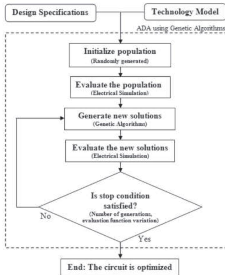
Fig. 2. Simulation-based design flow using genetic algorithms.
