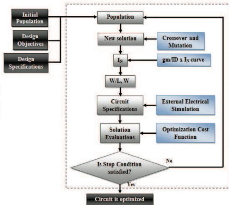
Fig. 4. Design flow for the  $gm/I_D$  design methodology.
