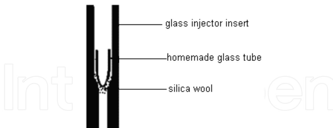
Fig. 5. The modified sample injection part of GC instrument. The dimension of the homemade tube: outer diameter, 2.0 mm; length, about 15 mm
