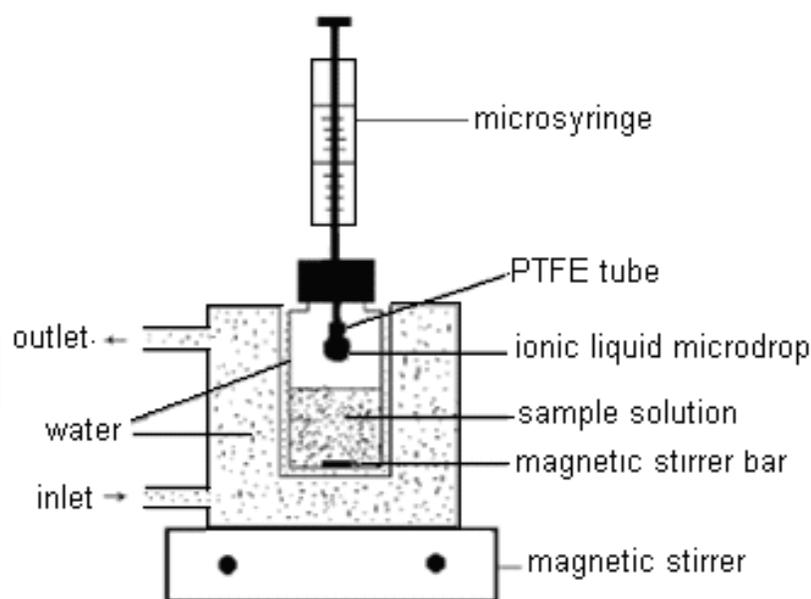
Fig. 2. Schematic diagram of SDME
