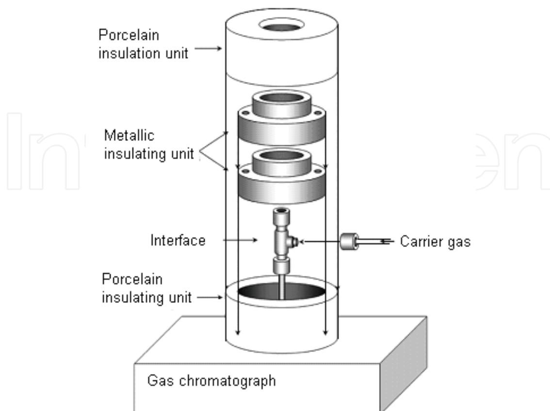
Fig. 4. Scheme of the household unit of the interface for the direct introduction of analytes extracted in a drop of ionic liquid into a gas chromatograph
