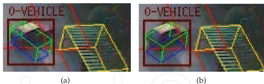
Fig. 4. Geometrically ambiguous solutions for the problem of associating a parallelepiped to a blob. Figure (a), shows an ambiguity between vehicle model instances, where the one with incorrect orientation has been chosen. In Figure (b), the correct solution to the problem.
