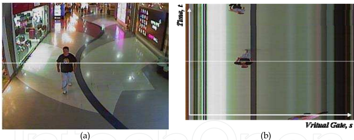
Fig. 1. (a) A virtual gate to measure pedestrian traffic size, (b) a spatiotemporal image created using the virtual gate
