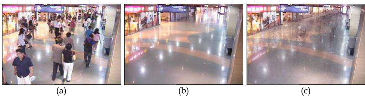
Fig. 4. (a) a scene with continuous pedestrian movements, (b) method clear background model under low human traffic, (c) a defected background model due to continuous movements of humans.
