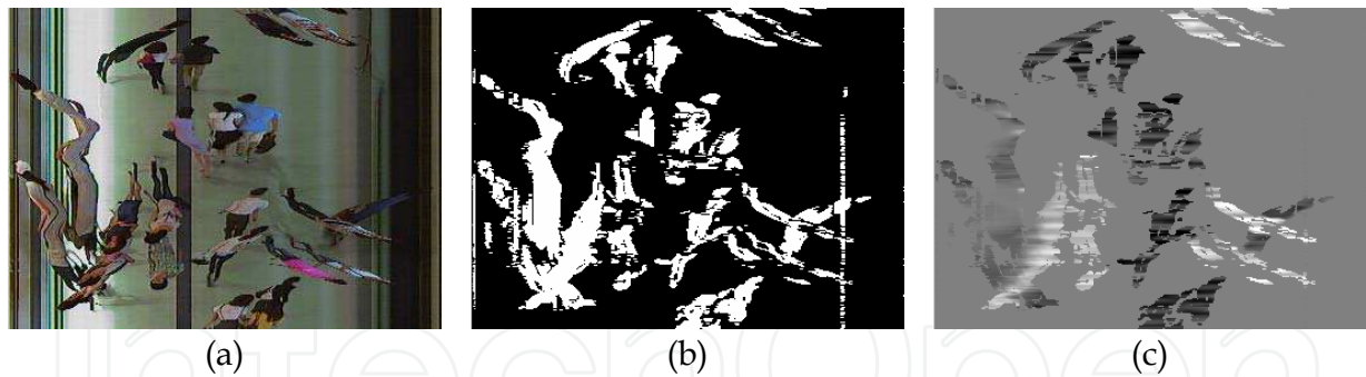
Fig. 7. Feature extraction results: (a) spatiotemporal image, (b) foreground map, (c) motion vector map
