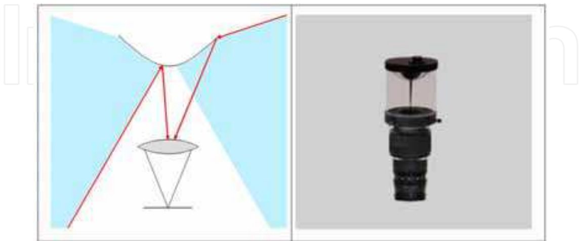
Fig. 3. Single mirror catadioptric optic. On the left the optic’s schema, on the right a catadioptric lens.
