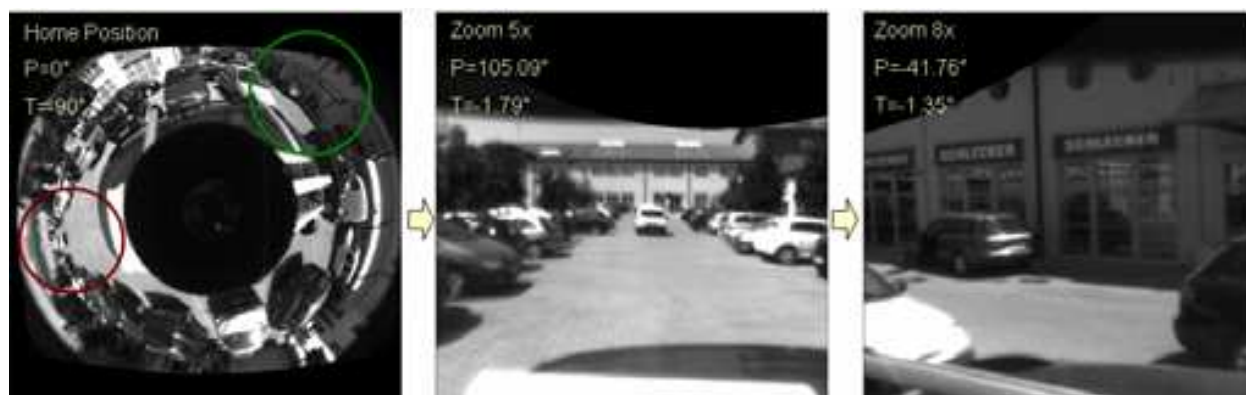
Fig. 15. Example of a virtual PTZ. On the left an image from a catadioptric lens mounted over a car. In the middle the projection of the area circled in red and on the right the projection of the area circled in green.
