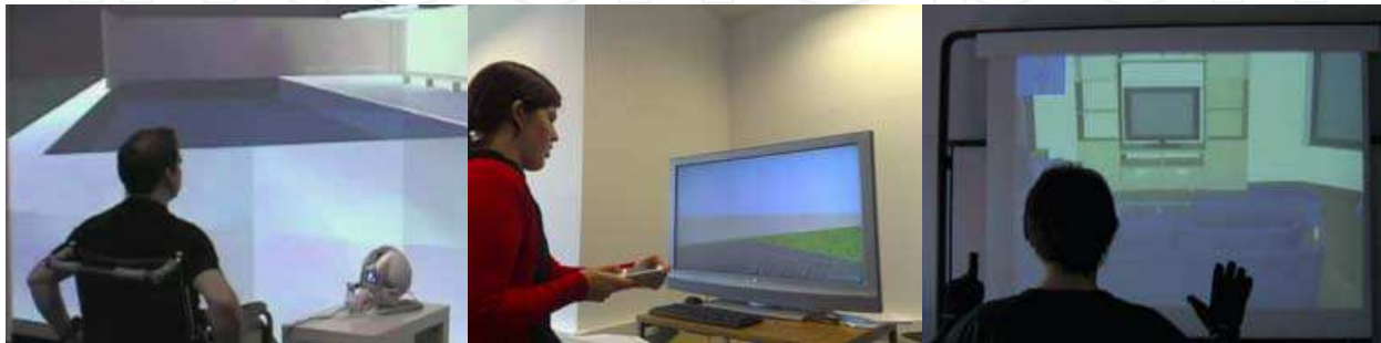
Fig. 7. Testing VR using a wheelchair and Falcon (left), smart phone (centre) and infrared data gloves (right)
