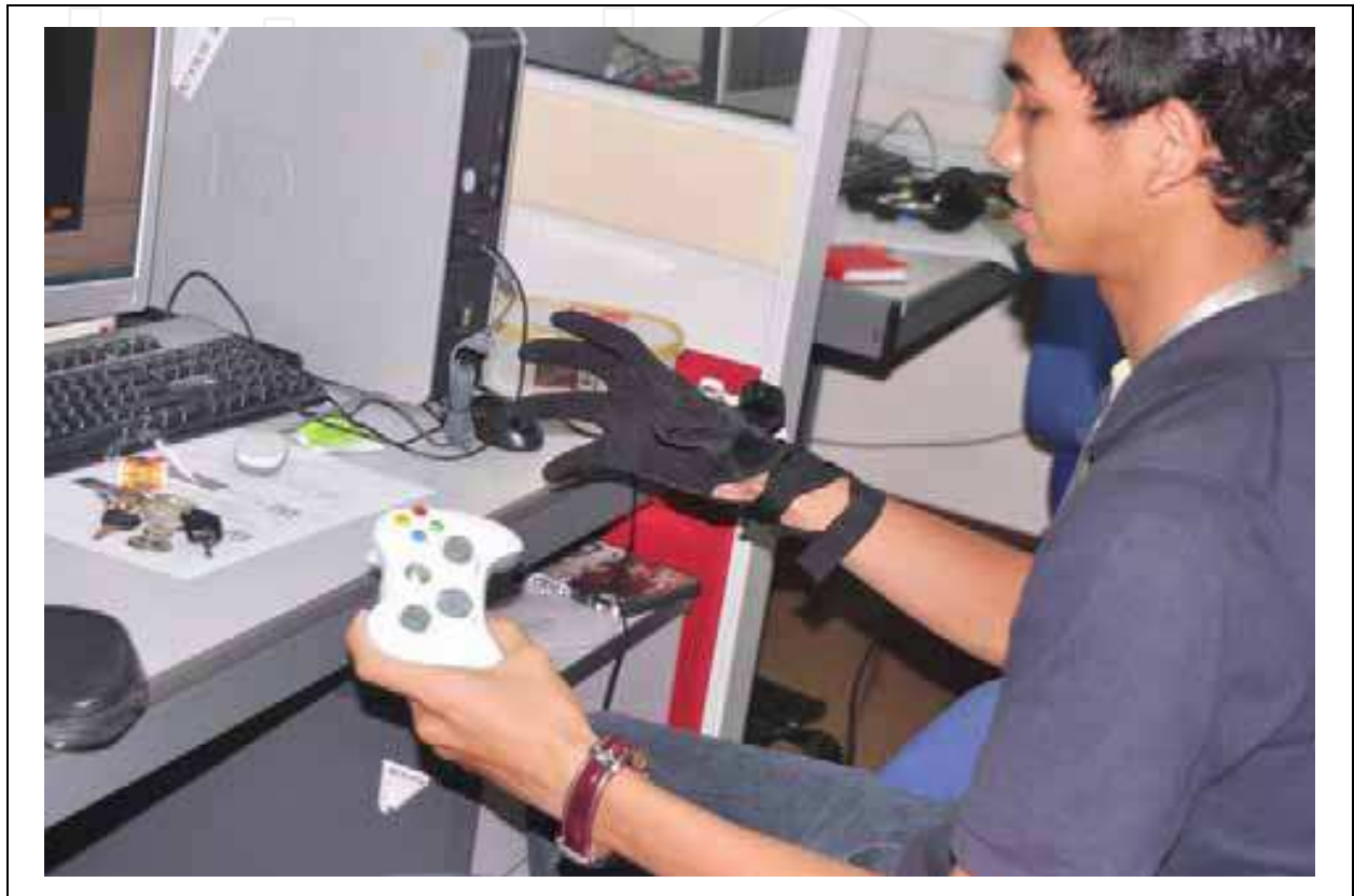
Fig. 9. User Interaction with avatar through XBOX windows controller and 5DT Data Glove-1
