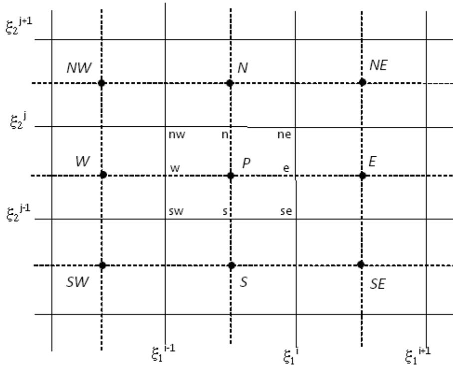
Fig. 2. Boundary condition treatment for finite volume method
