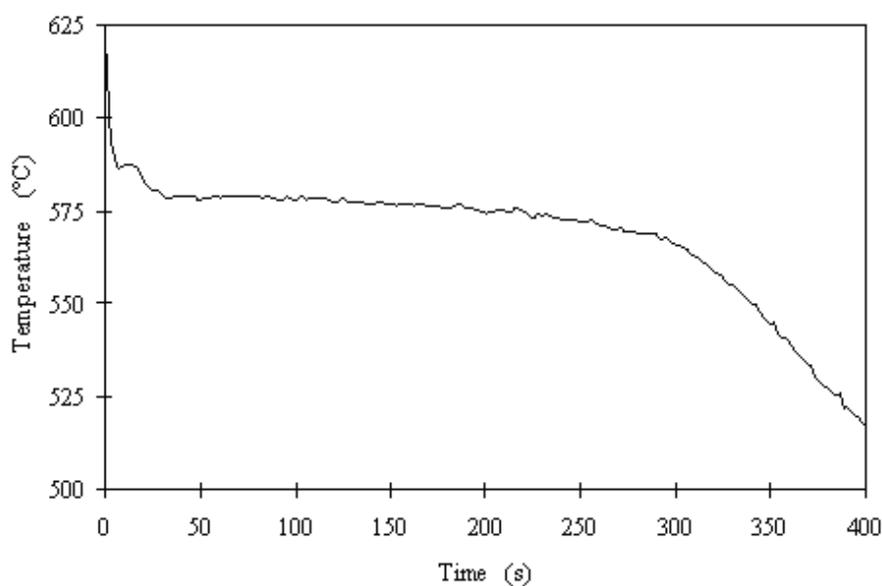
Fig. 7. Temperature profile during solidification of Al 12Si
