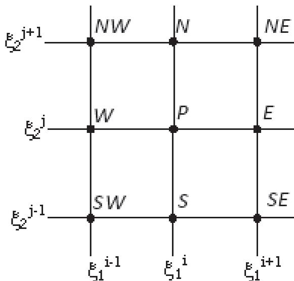
Fig. 3. Boundary condition treatment for finite difference method
