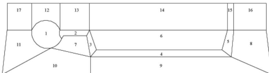
Fig. 9. Geometry division into 17 blocks
