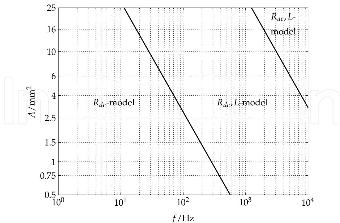
Fig. 8. Modeling guidelines: Based on the relevant frequency and the cross section of the wire, an adequate model can be selected.
