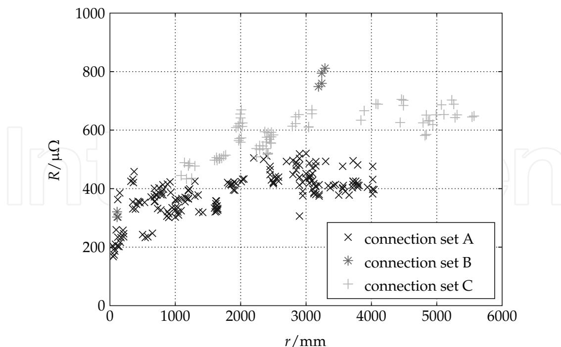
Fig. 11. Measured resistance between two grounding bolts. The resistance values are grouped according to the location of the grounding bolts.
