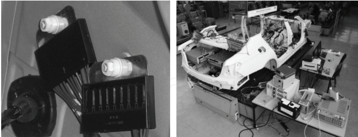
(a) The negative terminals of the components are connected to bus bars. Here, two bus bars are screwed to two grounding bolts that are welded to the car body.
