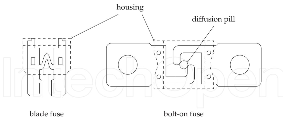
Fig. 9. For circuit protection, different kinds of fuses can be used. In the automotive wiring harness, the most common fuses are blade fuses or bolt-on fuses.
