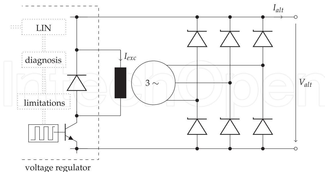
Fig. 5. Schematic of an automotive alternator. A voltage regulator controls the excitation of the electrical machine. The rectifier bridge converts the output of the electrical machine to DC.
