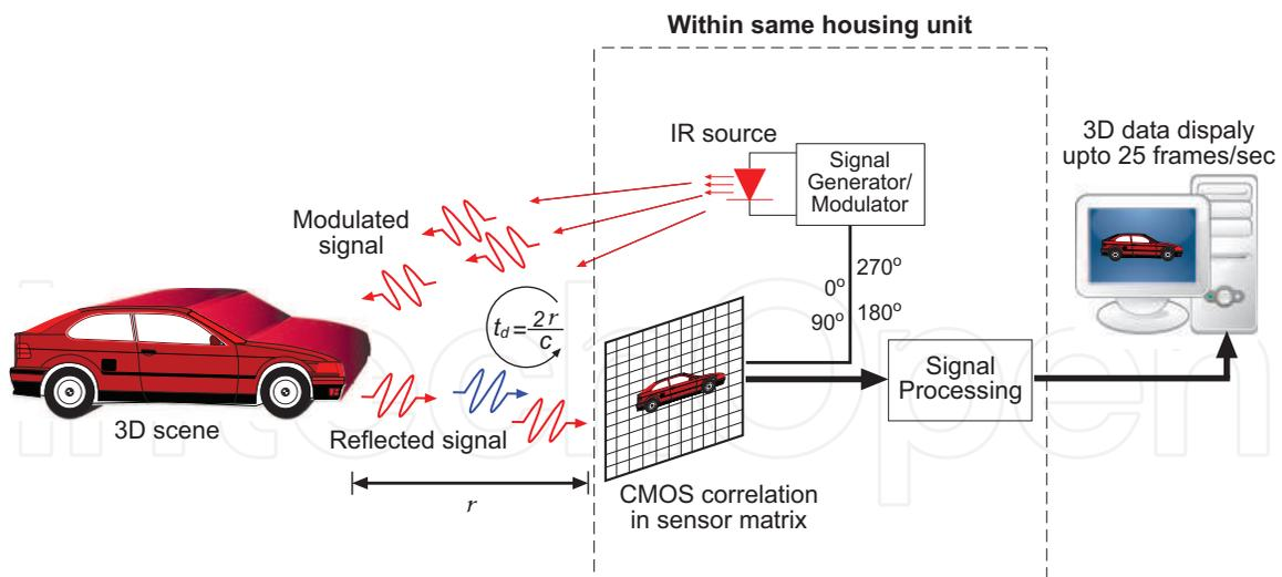
Fig. 2. Basic principle of TOF 3D imaging system.
