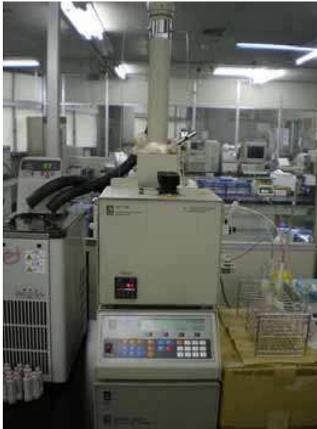
Fig. 2. Supercritical fluid extraction instrument used in this investigation
