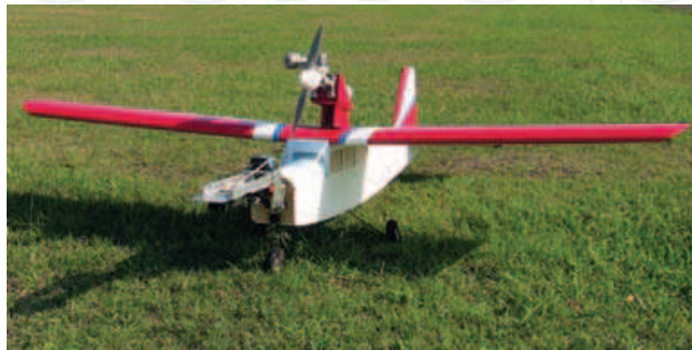
Fig. 7. The aircraft used for flight testing was a Super Frontier Senior-46 (wingspan 2040mm), modified so that the engine and propeller assembly is mounted above the wing.
