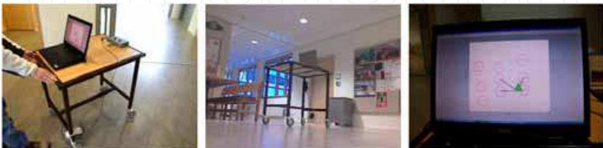
Fig. 20. Simultaneous localization and map building using only visual information at MDH. The table was moved at about 1m/ s producing the map of the room with 9 landmarks on a surface of about 50 m<sup>2</sup>
