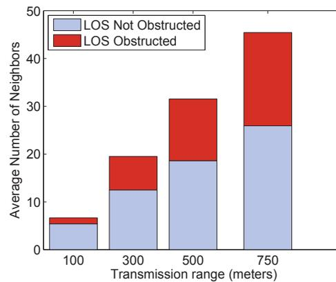
Fig. 7. Average number of neighbors with unobstructed and obstructed LOS on A28 highway. © [2011] IEEE
