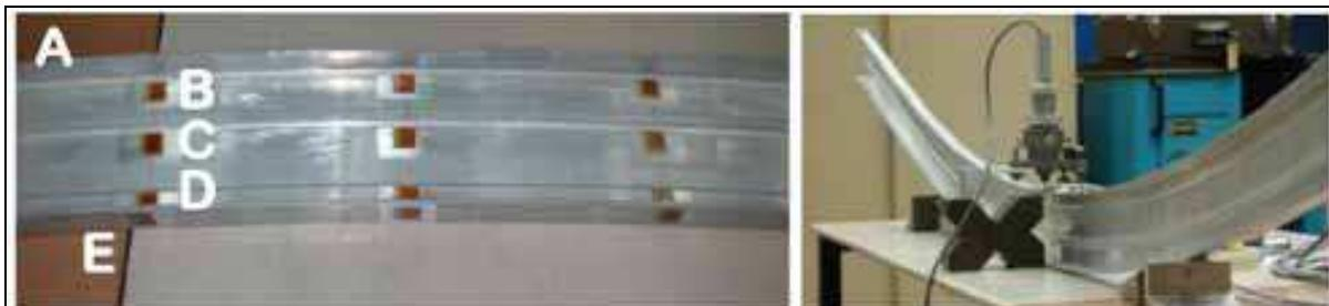
Fig. 13. Hole drilling measurement locations and test apparatus
