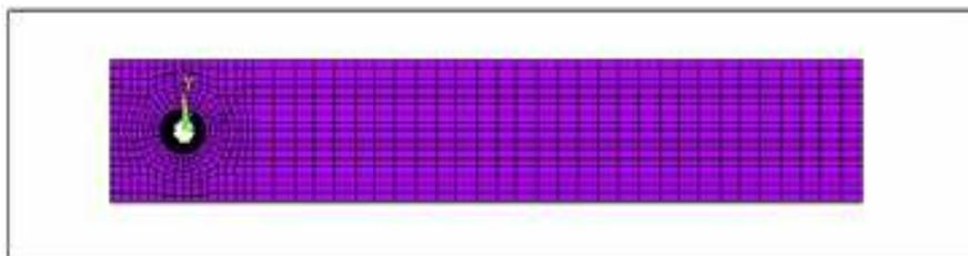
Fig. 9. FE model of a single joint sheet
