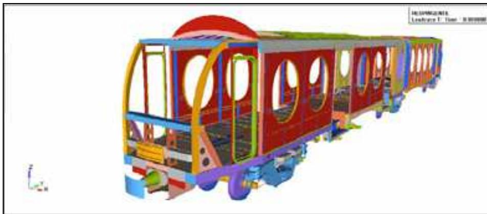
Fig. 21. The FEM model of a train coach
