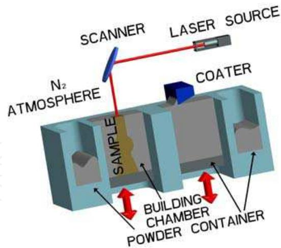
Fig. 1. SLM equipment
