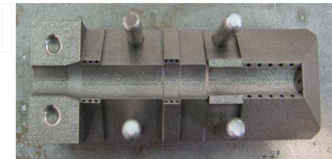
Fig. 15. Laser sintered lower component of the jig
