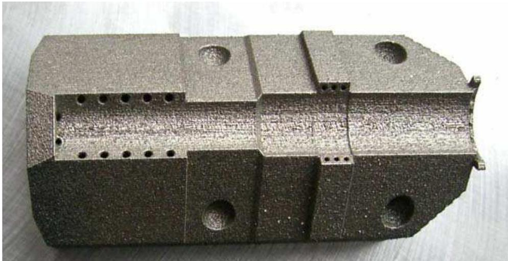
Fig. 14. Laser sintered upper component of the jig
