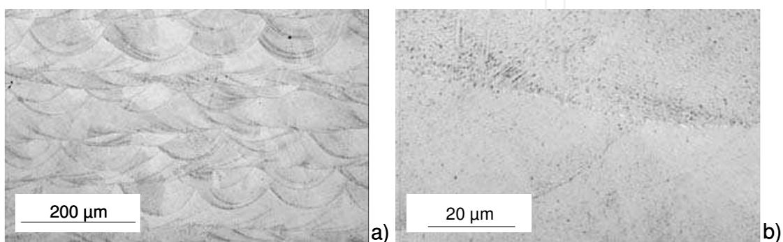
Fig. 4. 200x magnification (a) and 1000x magnification (b) of the sample obtained with  $P=100W$  and  $v=180mm/s$
