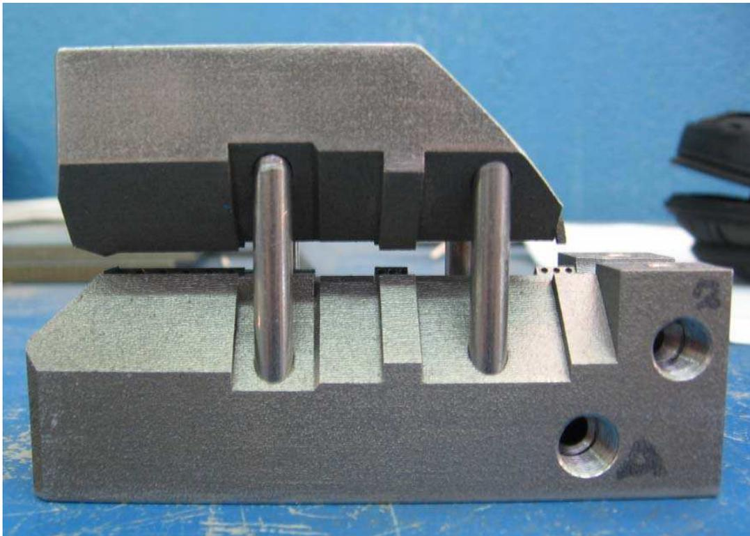
Fig. 16. Coupling of the jig components
