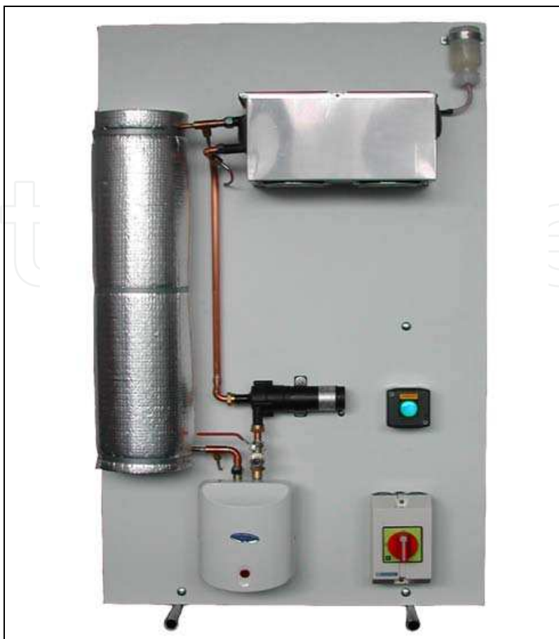
Fig. 15. Educational heating plant model with time-delay
