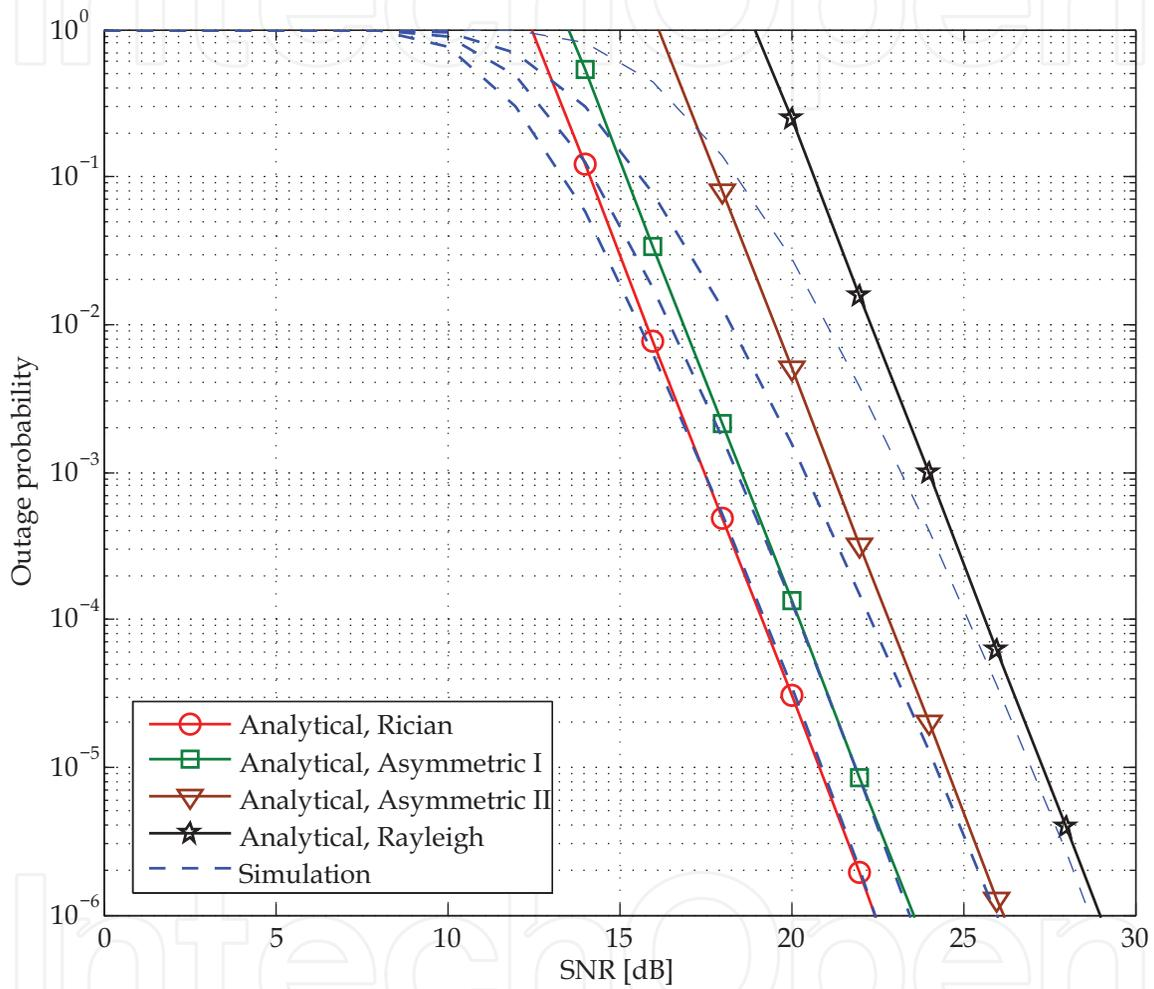
Fig. 4. The comparison of outage probability of repetition-based relaying over different fading channel such as Rician fading, Rayleigh fading, asymmetric channel I and asymmetric channel II. The number of relay nodes is of  $M = 5$ .
