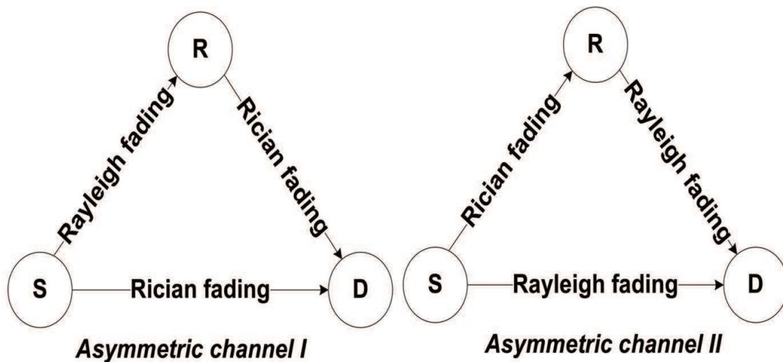
Fig. 1. Different asymmetric fading channels of a cooperative networks
