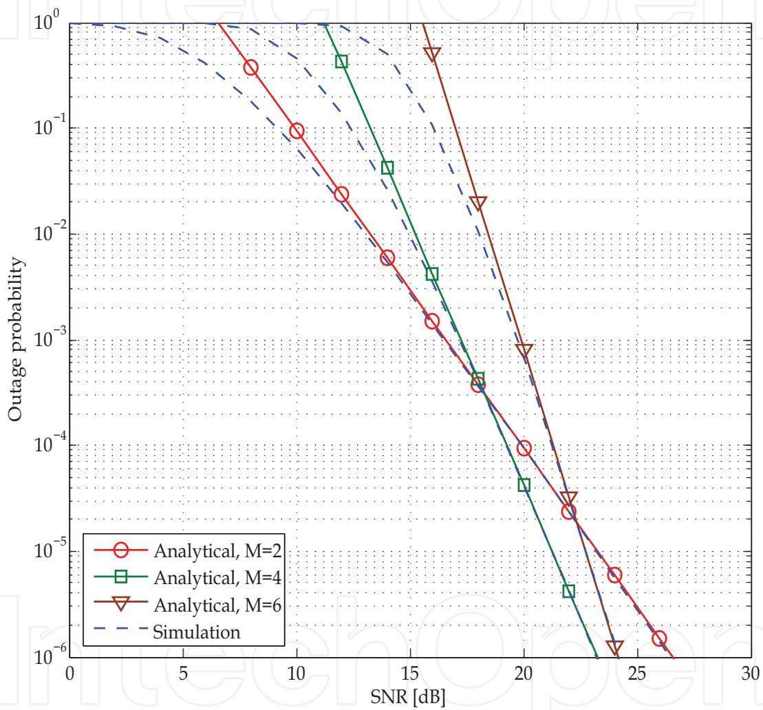
Fig. 2. The outage probability of repetition-based AF relaying over asymmetric channel I. The number of relay node is selected  $M = 2$ ,  $M = 4$  and  $M = 6$ .
