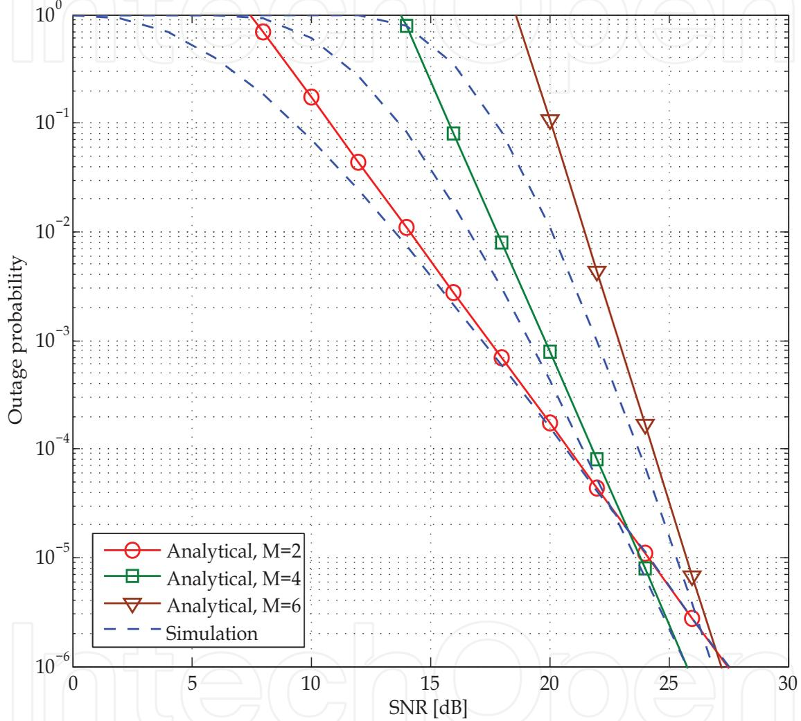
Fig. 3. The outage probability of repetition-based AF relaying over asymmetric channel II. The number of relay node is selected  $M = 2$ ,  $M = 4$  and  $M = 6$ .
