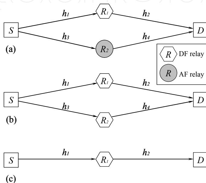
Fig. 8. hybrid DF-AF cooperation and DF cooperation architectures with different average power gains. (a) hybrid DF-AF cooperation, (b) dual DF cooperation, (c) single DF cooperation. ( $S$ : Source,  $D$ : Destination,  $h$ : average power gain between two nodes).
