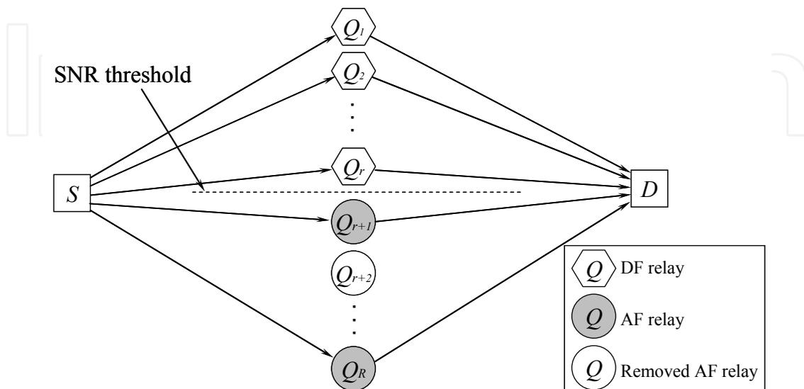
Fig. 3. Hybrid relay cooperation with dynamic optimal combination of DF-AF relays ( $S$ : Source,  $D$ : Destination,  $Q_r$ :  $r$ -th Relay)
