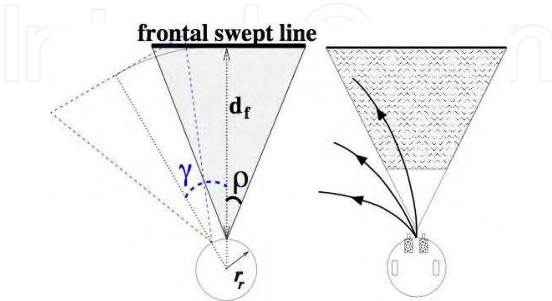
Figure 1. Problem formulation. (Left) The sensor Field of Regard is defined by three parameters: the field of view  $\rho$ , the depth of field  $d_f$ , and the field orientation  $\gamma$ . (Right) Tunnel vision problem: a fixed Field of Regard can be insufficient to sweep all the possible robot trajectories, with the corresponding safety risk
