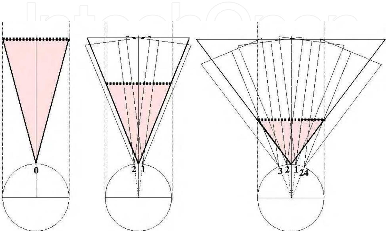
Figure 7. (Left) Virtual sensor implemented with a unique frontal ultrasonic sensor of aperture 15 deg. (Center) Virtual sensor implemented with two sonar sensors, located at  $\pm 7.5$  degrees from the main robot axis, robot B-21, aperture 22.5 deg. (Right) Virtual sensors implemented with four sonar sensors, located at  $\pm 7.5$  degrees from the main robot axis, robot B-21, aperture 37.5 deg
