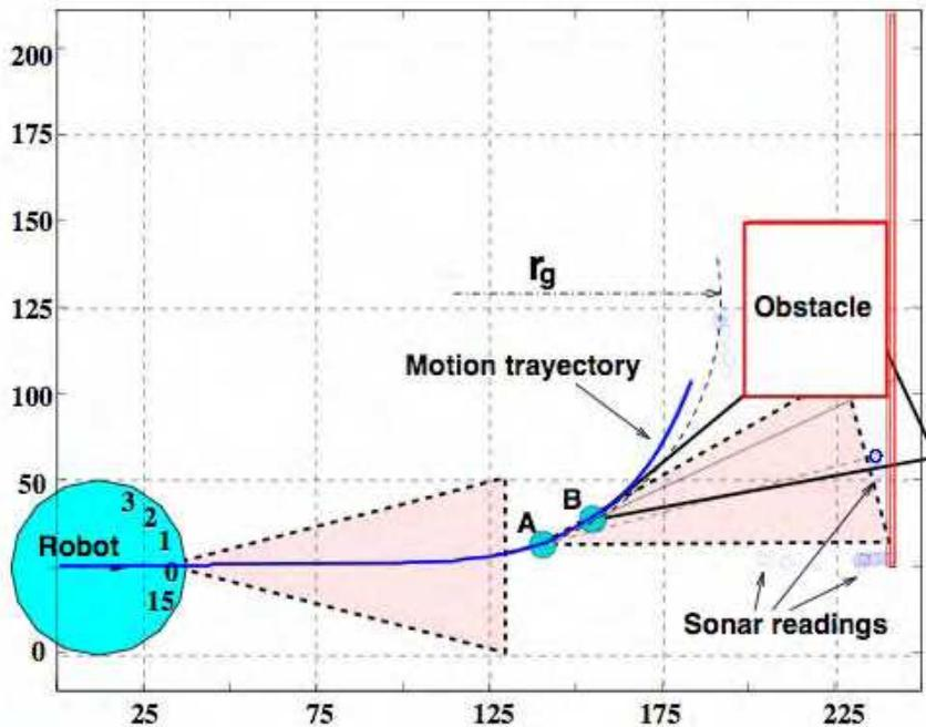
Figure 4. Stop maneuver triggered by an “ $A_2$  zone” obstacle in a real experiment; top view. From point A to point B the robot is turning at maximum speed, and the sensor is measuring a maximum distance  $d_f$ ; in B the obstacle corner comes into view, and an abrupt range measure is read, leading to an emergency stop condition (and eventually a collision)
