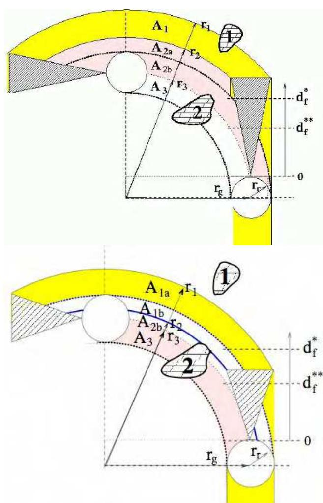
Figure 3. Robot turning with constant velocities. Its sensor Field of Regard fulfills conditions (4) and (6). (Left) Case when  $d_f > d_f^*$  and the tunnel vision problem: the robot moves where the sensors did not reach. (Right) For  $d_f^{**} > d_f > d_f^*$  the situation is better, but still there are blind zones
