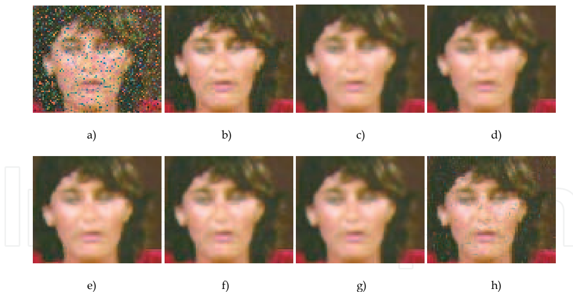
Fig. 4. a) Zoomed image region of 10th Miss America frame contaminated by impulsive noise of 15% intensity, b) Designed 3D-FCF, c) 3D-MF; d) 3D-VVMF, e) 3D-VGVDF, f) 3D-VAVDATM; g) 3D-VATM; h) 3D-VKNNF.
