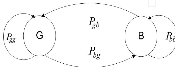
Fig. 2. Lutz's Two-state LMS channel model.
