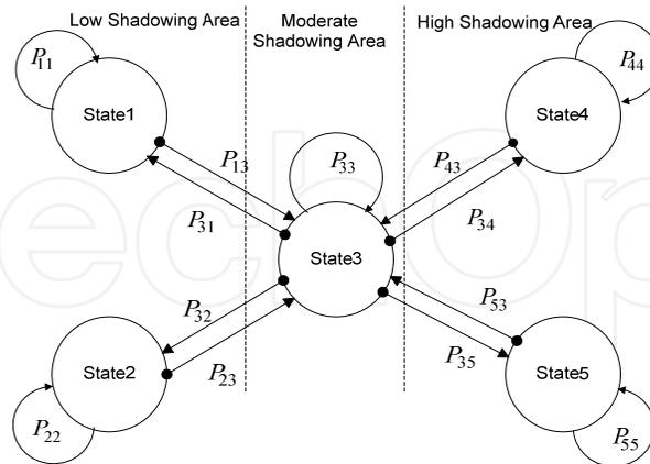
Fig. 4. Five-state Markov channel model for LMS communications.
