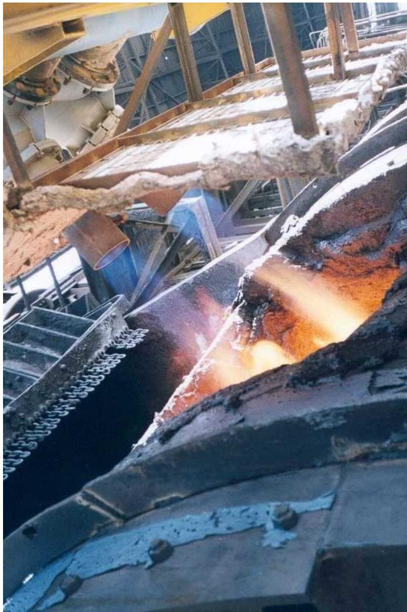
Fig. 7.1 Photo of Burners Installed in P&S Furnace
