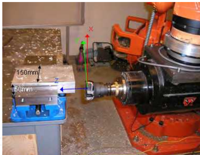
Fig. 6. Robotic end milling process setup
