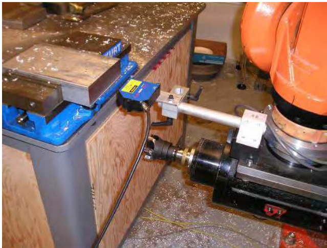
Fig. 16. Setup of aluminum end milling and surface scan
