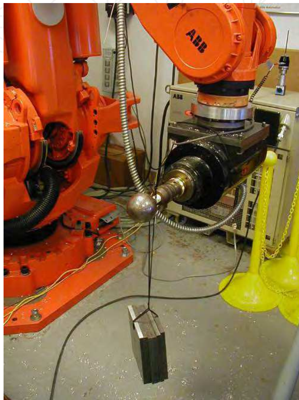
Fig. 14. Methodology of robot stiffness measurement
