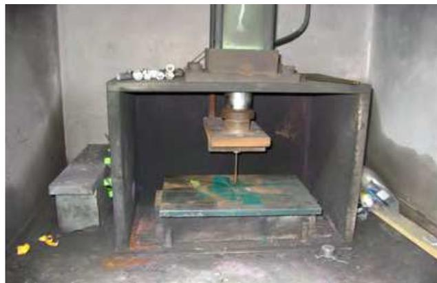
Fig. 1. Nail penetration Test equipment.
