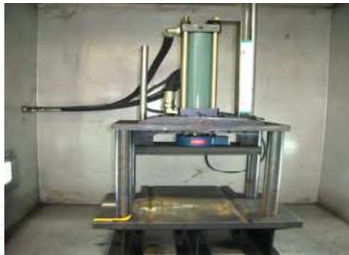
Fig. 2. Impact test equipment
