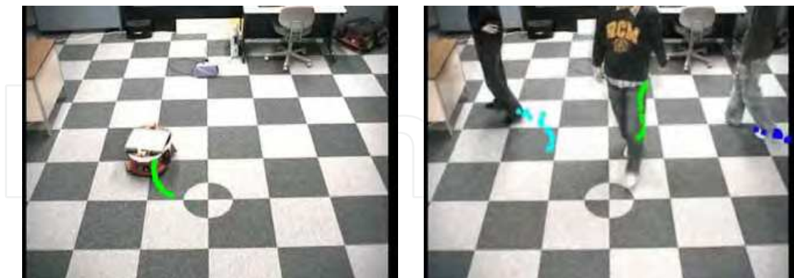
Fig. 5. Examples of mobile robot tracking and multiple people tracking using three laser range finders. The tracking results obtained in a position server mentioned below are overlaid on video images.
