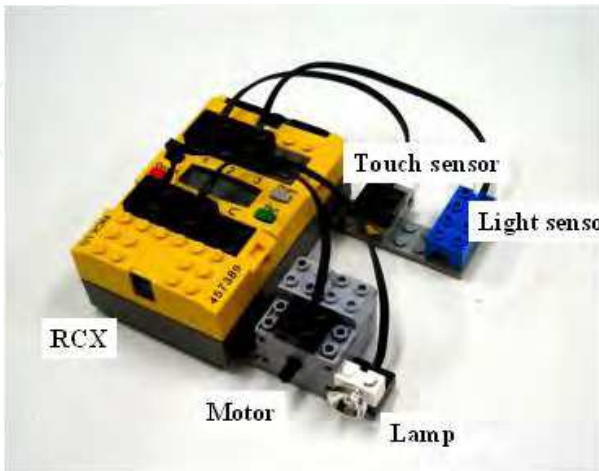
Fig. 6. A configuration of RCX, which connects with actuators and sensors.
