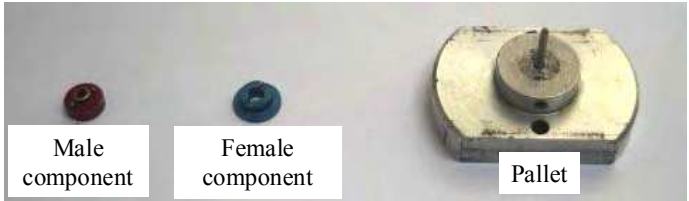
Fig. 4. A pair of components and pallet used in the miniature automated production line
