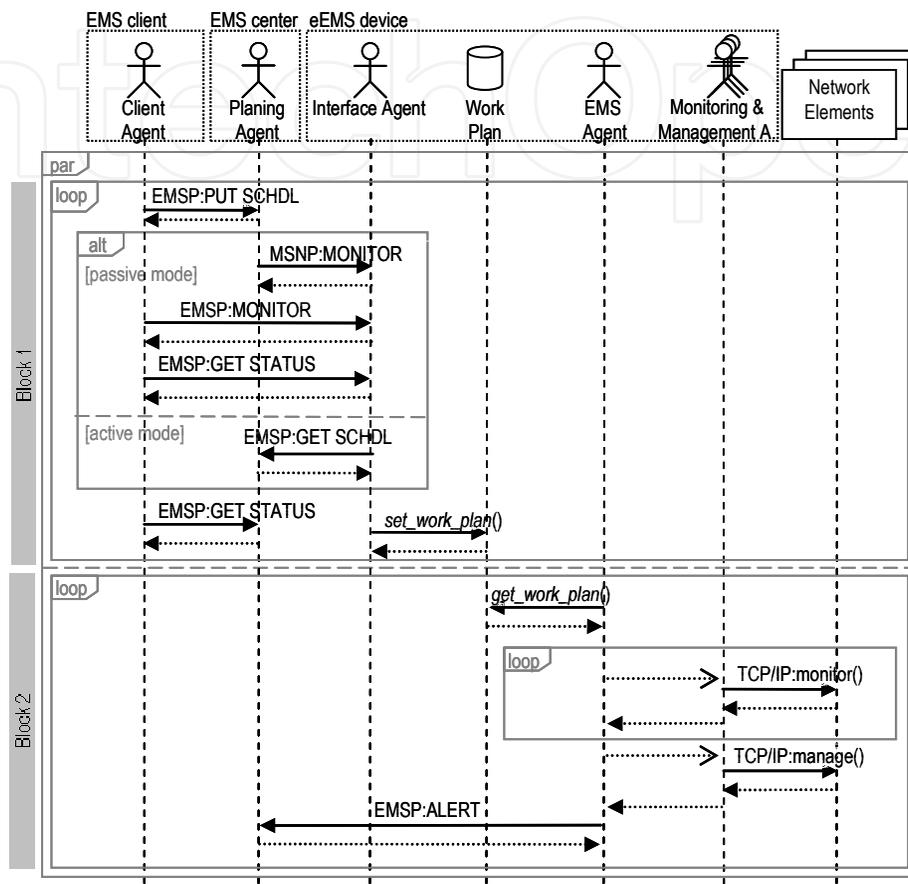
Fig. 3. Sequence diagram of the EMS main functionality.
