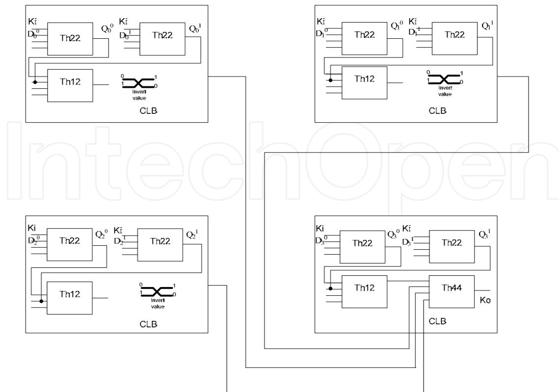
Fig. 16. 4-bit NCL register implemented at level-2 structure.
