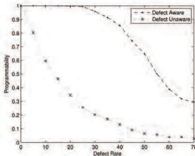
Fig. 20. Programmability comparison for defect-aware and -unaware approaches
