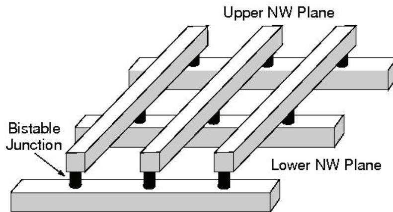
Fig. 1. Typical nanowire crossbar architecture
