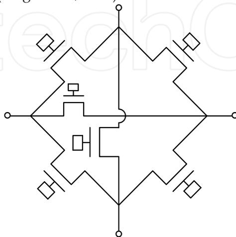
Fig. 17. Six Pass Transistors Interconnects (Lee et al., 1999).
