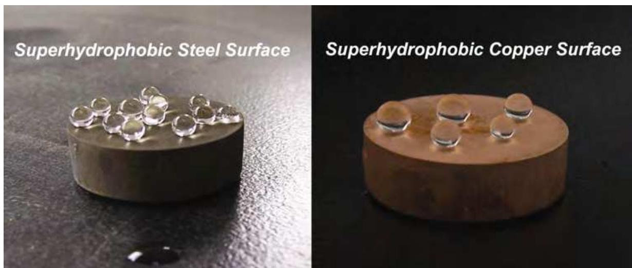
Fig. 8. Image of water droplets with different sizes on the superhydrophobic surface of steel having a contact angle of  $161 \pm 1^\circ$  and on the superhydrophobic surface of copper alloy with a contact angle of  $158 \pm 1^\circ$  respectively (Qu et al., 2007). (Reproduced with permission from Wiley-VCH Verlag GmbH & Co. KGaA, Copyright 2007.)
