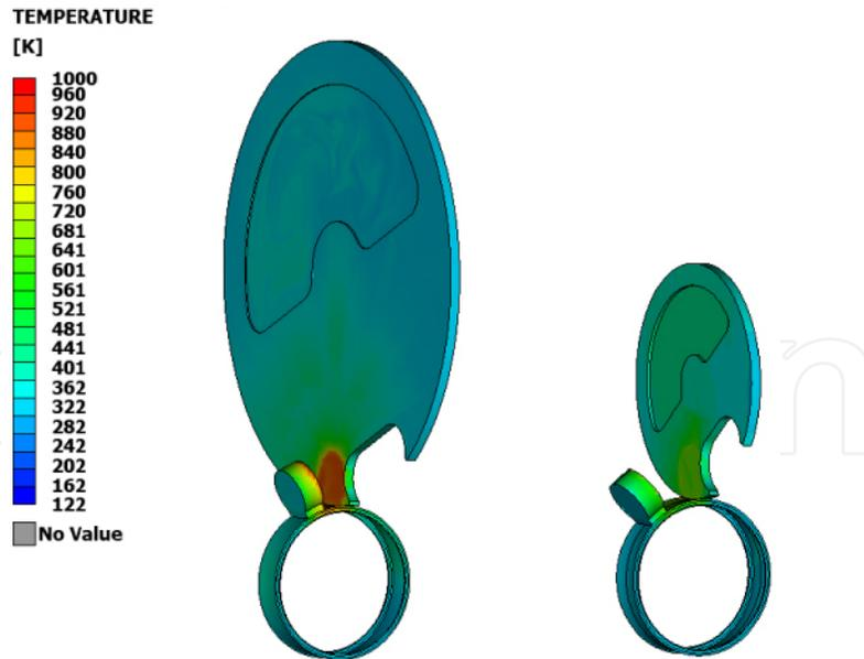
Figure 26. Temperature distribution for both RSP sizes.
