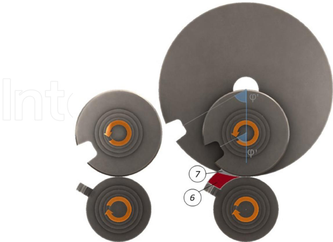
Figure 4. SARC with the nominal (left side) and double RSP diameter (right side).
