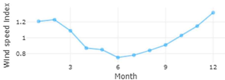
Figure 7. Normalized wind speed at the new turbine location using Global Wind Atlas Online Software.
