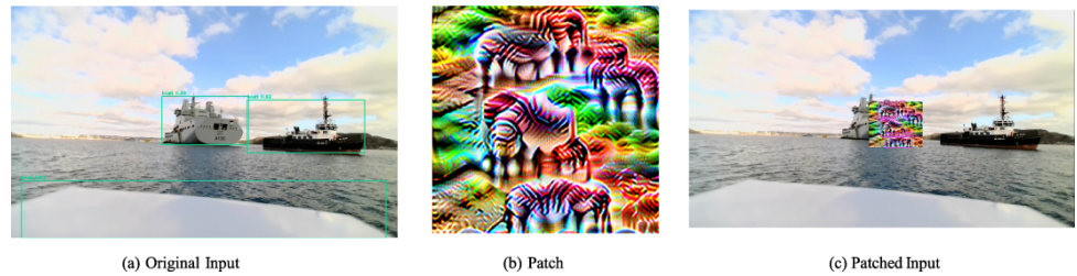
Figure 4. A real-world adversarial patch attack sample [56] generated to attack the common pre-trained YOLOv3 object detection model. The input sample, an image of two vessels, is predicted as a vessel by the model, providing a confidence value of 99% and 92%. An adversarial patch (b) is provided digitally or physically (e.g., as a sticker) to change the detection prediction to a zebra by the model. Notice the patch can interfere with the prediction and hide nearby objects, such as the second ‘boat’, i.e. vessel, on its right in the photo. The patch does not need to be significantly large but can be closer to the camera than the evading objects to produce the desired effect.
