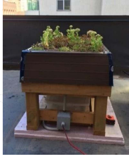
Figure 6. Green roof test module with reservoir to capture run-off and load cell instrumentation to obtain evapotranspiration values.
