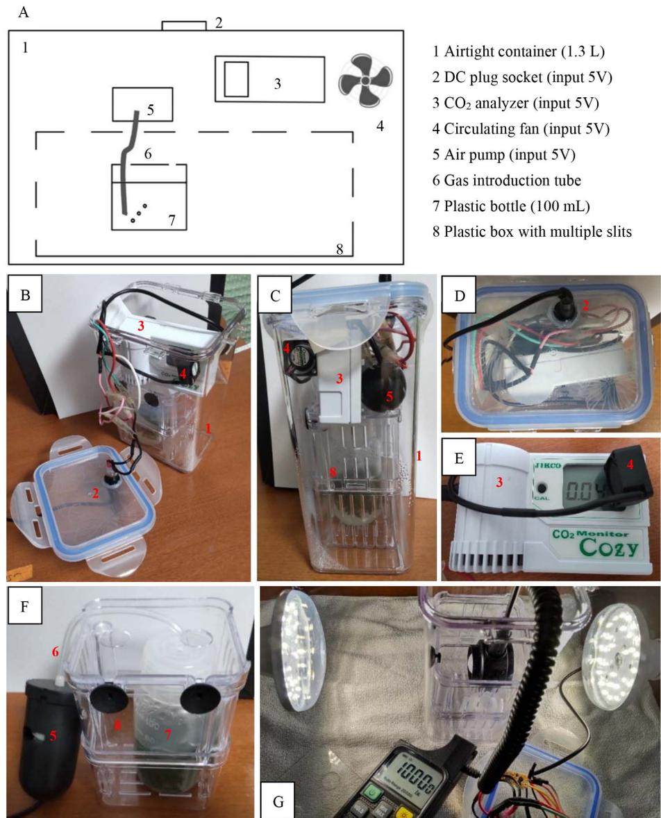
*Figure 3.* CO<sub>2</sub> analysis system in a closed small-space. (A) Schematic diagram. (B) General view. (C) Lateral view. (D) Top view. (E) CO<sub>2</sub> analyzer and circulating fan. (F) Air pump and gel-containing bottle in a plastic box with multiple slits. (G) Adjustment of light intensity of the white LED lamp using a digital light meter.
