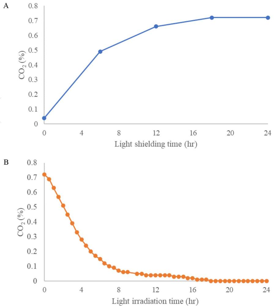
Figure 4. Measurements of (A) CO<sub>2</sub> production by CO<sub>2</sub> generator and of (B) decarboxylation by SGG in a closed small-space of CO<sub>2</sub> analyzing system.  $N = 3$ .
