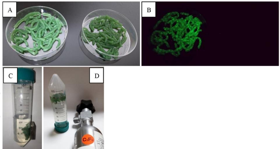
*Figure 2.* SGG containing each functional material. (A) Phosphorescent (*left*) and regular (*right*) SGG. (B) Light emission of light-irradiated phosphorescent (*left*) and regular (*right*) SGG in the darkroom. (C) Magnetic separation of SGG containing iron powder. (D) Flotation separation of SGG containing C<sub>3</sub>F<sub>8</sub> gas.
