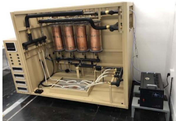
Figure 4. Testing rig of the microchannel heat sink.
